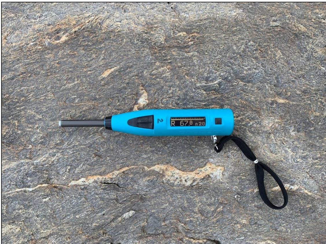
*Figure 3. 2: Image showing the digital N-type Schmidt hammer used in this study, specifically, the ‘Rockschmidt’ manufactured by Proceq in Switzerland. Source: Author.*
