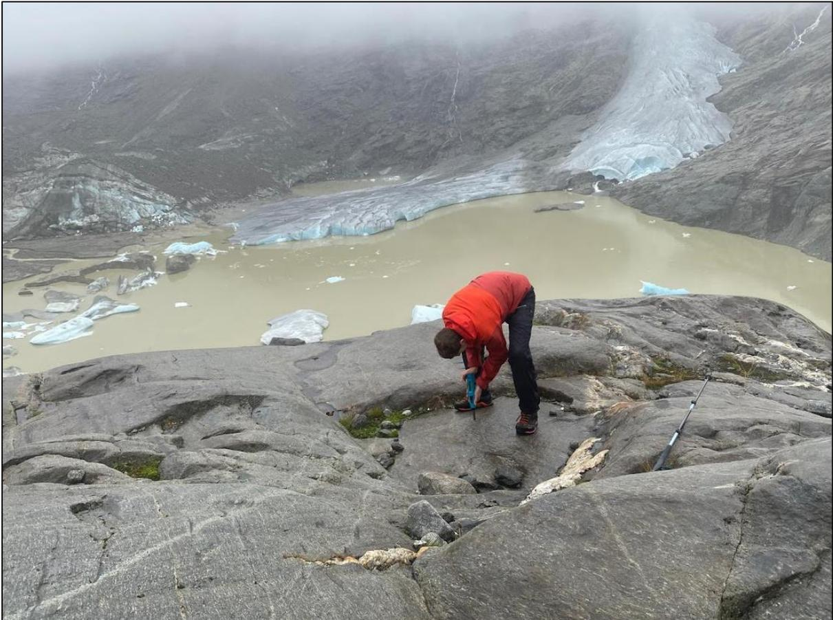
*Figure 3. 3: Image showing the author applying the Schmidt hammer to a section of bedrock at a perpendicular angle. Source: Author.*
